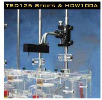
istics and excellent linearity. The transducers come with a versatile mounting rod assembly to support a variety of orientations. When fine tension and position adjustments are required, clamp the mounting rod to an HDW100A (see below).
