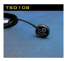
Use the TSD108 with the NEW EBI100C Electrical Bioimpedance amplifier for cardiac output measurements — see page 60.
