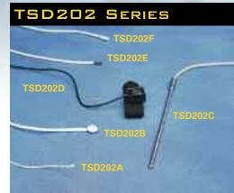
**Digit Surface Probe-** The TSD202D records skin temperature of the fingers or toes. The probe contains a surface temperature sensing element encased in a polyurethane housing that conforms to curved skin surfaces and includes a stretchy  $Velcro^{\$}$  strap for easy attachment.
