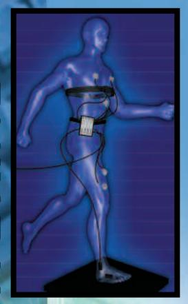
To increase subject comfort and minimize cumbersome wiring, use the TEL100C Remote Monitoring Module set. Each 4-channel module connects to the subject via a single thin coaxial cable. Cables are available to span from 10 to 60 meters between the subject and the MP System. Add remote monitoring module sets to an existing MP System to take tethered ambulatory measurements or to record from multiple, separated subjects.
