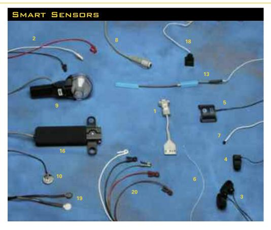
Smart Sensor (SS) electrodes and transducers connect to the TEL100M-C amplifier/transmitter. Any Smart Sensor electrode or transducer can be plugged into any TEL100M-C input. The following SS series transducers connect to the TEL100C system. The transducer specifications mirror the characteristics of the respective "TSD" types listed. Generally, biopotentials and other signals can be recorded for up to 24 hours. All transducers come with a 1.8-meter cable unless otherwise specified.
