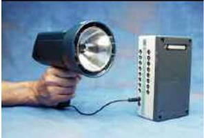
data acquisition. The TSD122 is battery-operated and will operate from zero to 12,000 flashes a minute. Cables are included for interfacing with the MP System.
