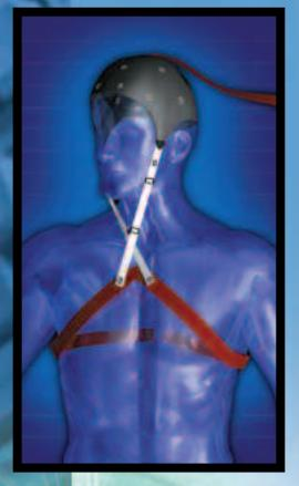
Record up to 16 leads and use the on-line software features to derive new leads or filter raw data for a wide range of EEG applications on human and animal subjects. For example, set up multiple-lead unipolar or bipolar montages, or emphasize changes in occipital lobe alpha activity as a consequence of experimental procedure. A variety of stimulus/response protocols are possible when using the averaging options and stimulator accessories.
