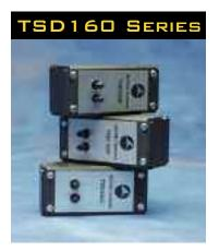
The TSD160 series differential pressure transducers are designed for low range pressure monitoring. The transducers plug directly into the DA100C general-purpose differential amplifier. The differential pressure ports are located on the front of the transducers and are easily connected to breathing circuits, pneumotachs or plethysmograph boxes. These transducers are very useful for interfacing a
