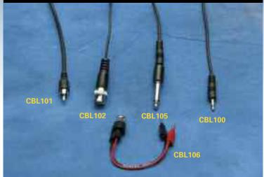
The CBL106 is a multi-purpose adapter used in conjunction with the CBL102 to connect a BNC cable to the digital I/O lines on the UIM100C or to the input of the DA100C. It also connects the STM100C to nerve conduction chambers (CBL102 required).
