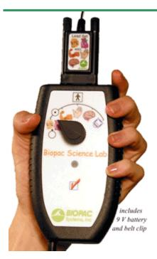
Measurements: ECG, EEG, EOG, EMG (high level), EMG (low level)
