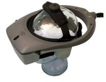
HMD2 is a state-of-the-art head-mounted display (HMD) for advanced virtual reality applications. It incorporates high-resolution color microdisplays with custom engineered optics to deliver unsurpassed visual acuity in a wide field-of-view format.
