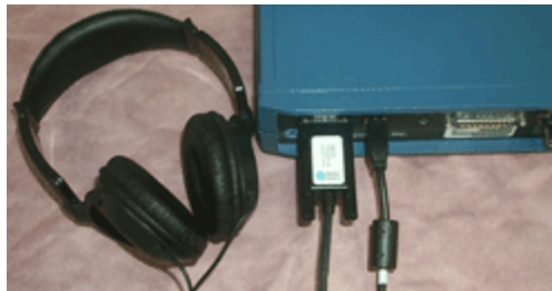
OUT1 plug into back of MP35 unit for auditory biofeedback
