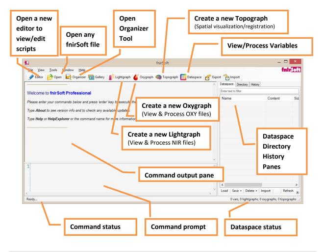
Below is the main window of fnirSoft with common user elements and tools identified.
