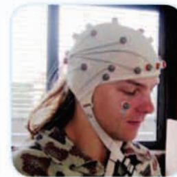
Conventional EEG cap & electrodes
