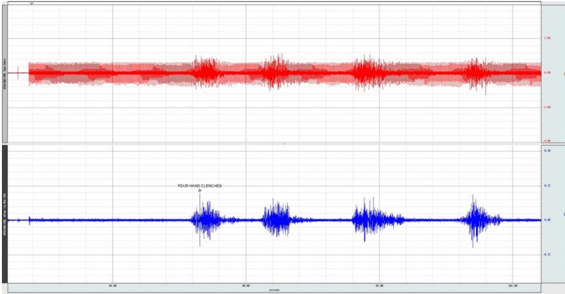
In this graph, a close-up is provided of the EMG data, right after the start of scanner EPI. Note the very clear “outline” of the EMG data in the first (red) waveform. The second waveform simply extracts this data using a basic CBS filter.
