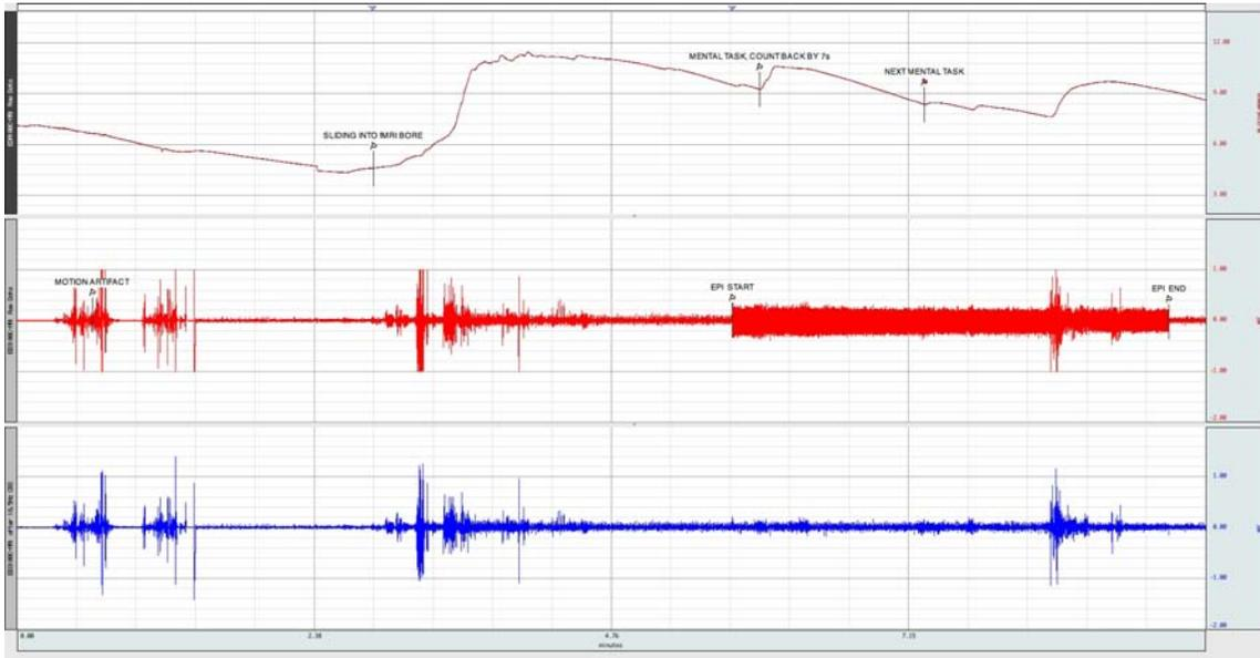
The top waveform in the graph is the raw electrodermal activity (EDA) data obtained from the EDA100C-MRI, set to a gain of 5 uS/Volt, DC coupling set to ON and 1 Hz LP set to ON. Electrodes were connected to the index and middle finger of the subject, so as to record standard EDA. Note that the top (red) waveform is unaffected by the advent of EPI.
