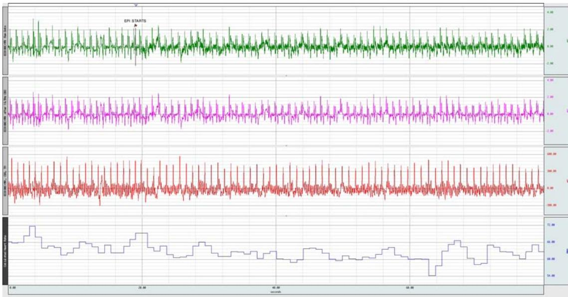
The top waveform in the graph is the raw electrocardiogram (ECG) data obtained from the ECG100C-MRI, set to a gain of 1000, with 1 Hz HP set to ON and 35Hz LPN set to ON. Electrodes were connected to the chest of the subject, so as to record a LEAD II ECG. Note that the top (green) waveform is relatively unaffected by the advent of EPI, in that R waves are clearly identifiable.
