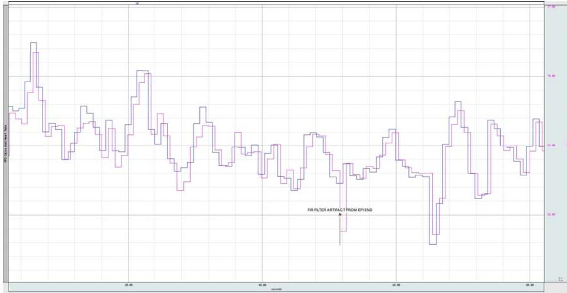
The data in this graph illustrates an overlap comparison of the rate (BPM) data derived from a PPG100C-MRI amplifier as compared to BPM data derived from a ECG100C-MRI amplifier. Both the PPG data and ECG data were collected, on the same subject, at the same time. Note that the derived BPM results are very similar, excepting one point which is a result of switching artifact when the 10Hz LP filter on the PPG100C-MRI amplifier was switched to 3 Hz LP.
