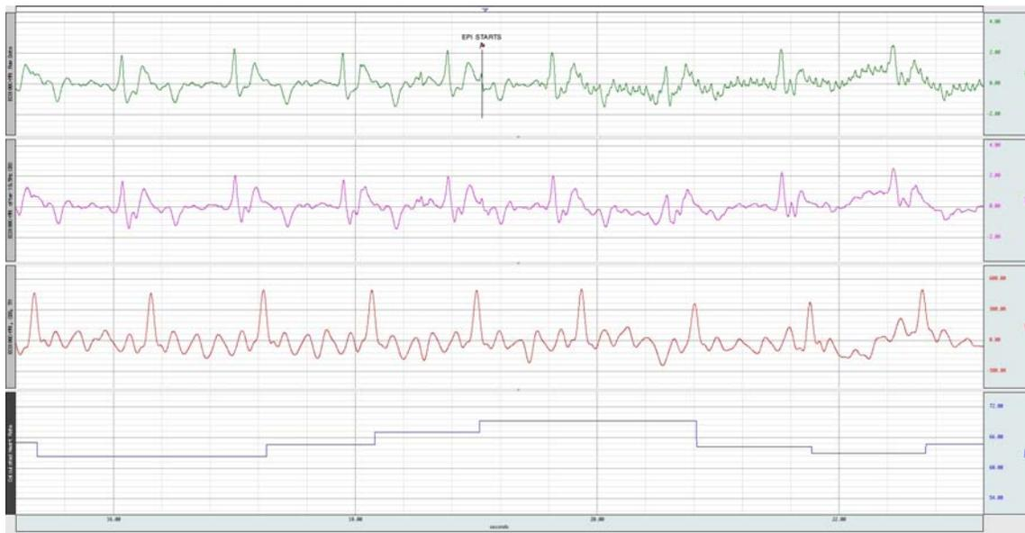
In this graph, a close-up is provided of the ECG data, right around the start of scanner EPI.
