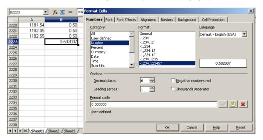
• The number obtained in this example is 0.502007 seconds between sample points. Write the result down as it will be required when importing data in Acq*Knowledge*.
