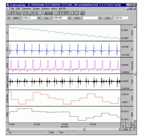
**dZ/dt**<sub>(max)</sub> is shown fifth from top and is being determined on a cycle by cycle basis from the raw **dZ/dt** waveform shown third from top.
