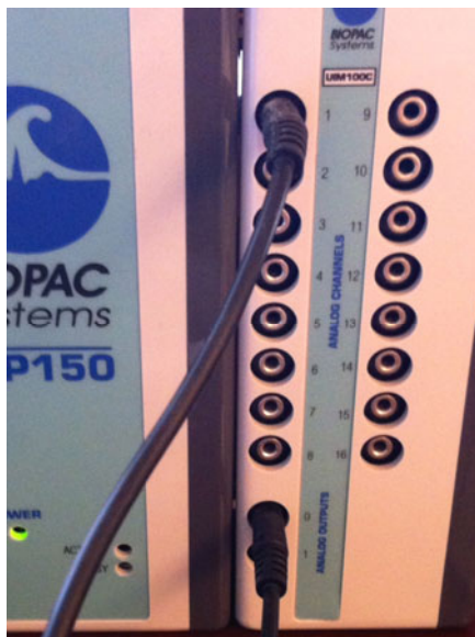
Analog Output 0 connected to CH 1
