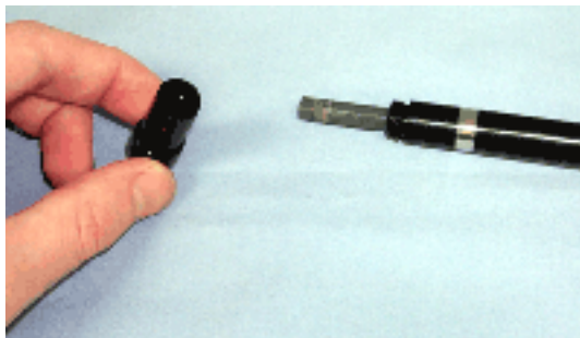
Unscrew the tip to fill/empty the electrolyte solution
