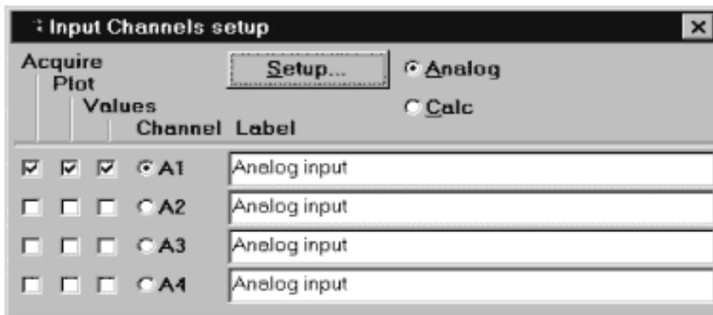
Select the **Setup** button, click on the **Presets** and highlight **EMG**. This will transform the universal amplifier into an EMG amplifier to give you the raw
