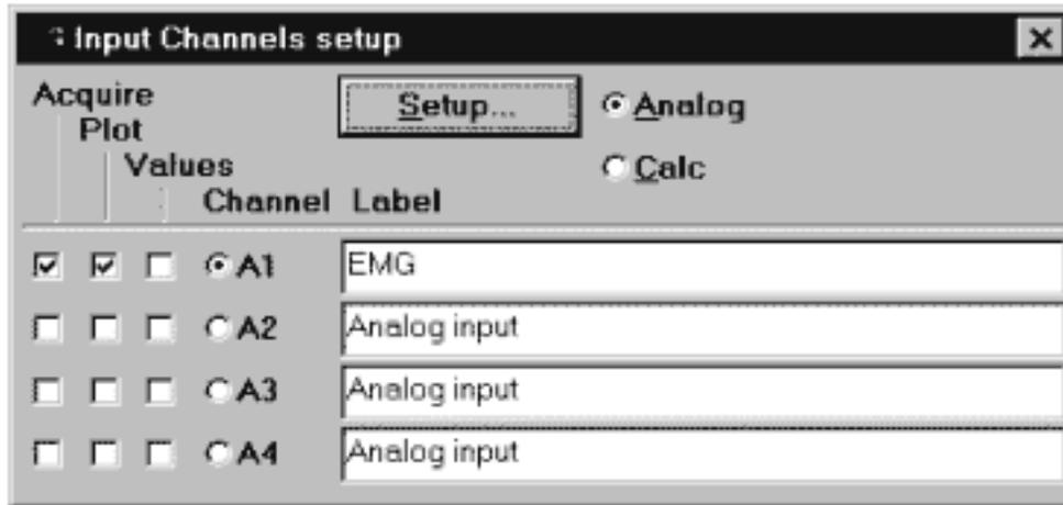
In order to obtain the integrated EMG, you must enable a Calculation channel and set it to Integrate. To do this you must click on the **Calc** button in the Input Channels setup box. Change the label from Calculation to Integrated EMG. Then check the Acquire, Plot and Values boxes and set the right-hand box to **Integrate**, as shown below.
