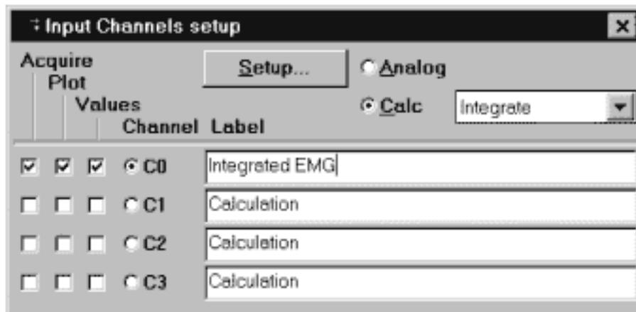
Finally, click on the **Setup** button, set the source to A1, samples to 20 and click on **Rectify first**. The samples value will vary, depending on the sample rate and time constant ( use 20 for 200 samples/sec and use 100 for 1000 samples/
