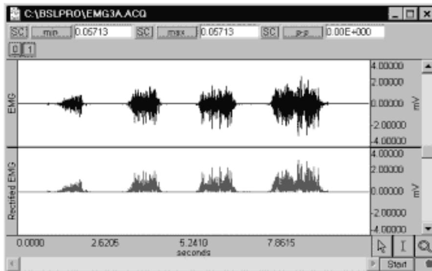
Finally, select **Smoothing** from the **Transform** menu and set the samples to 100, as shown below.
