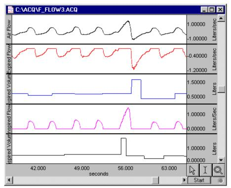
Expired lung volume can be recorded with some adjustments to the Rate calculation. From the Rate setup menu, select the appropriate calculation channel as the source and select Area from the Function menu. To calculate the area of the negative going waveform, use a Positive Polarity. Set the Peak Interval Window to suit the subject's respiration rate (human at rest: 5 and 25).
