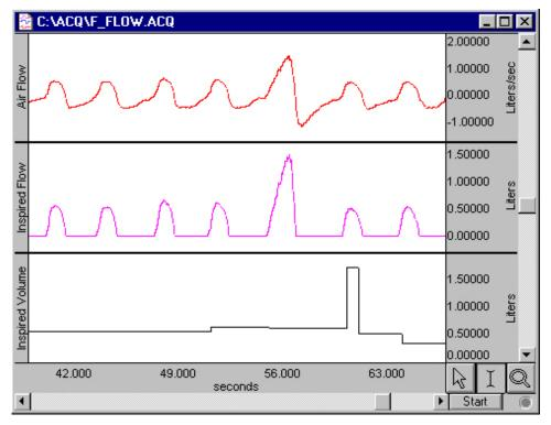
Expired volume can also be determined by adjusting the Limit settings. Set the Lower limit threshold to 0 liters/sec and the Upper limit threshold to -2.0 liters/sec. The upper limit must be set to a number greater than the most negative deflection of the signal (peak expired flow). Adjusting the Limit threshold cuts off the positive portion of the signal and leaves the negative part.
