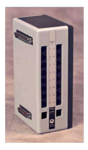
The HLT100A module is used to interface all high level output transducers to the MP100 system. The HLT100A module provides 16 input and 2 output channels. The HLT100A is similar in function to the UIM100A Universal Interface Module, but it also provides power to the transducer when making a connection. Connections to the HLT100A are made via a standard 6 pin RJ11 type connector.
