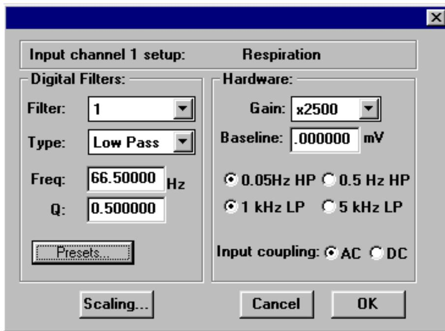
You may change the filter settings, in the same Setup window by clicking on or off the appropriate filter. You may use the same guidelines for filtering as above. The gain setting is set for a human recording, if your subject is much smaller you can adjust the settings by clicking on the Gain box.
