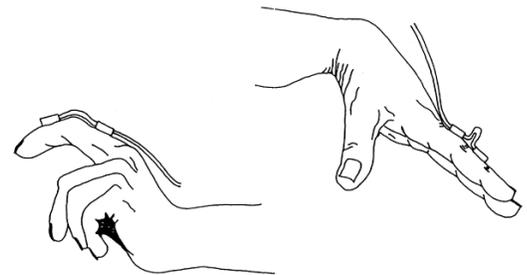
The unit is designed to fit over the joint to be measured and has extremely high flexibility to ensure the instrument does not interfere with normal joint movement. One endblock is attached either side of the joint.
