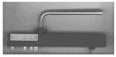
The TSD105A/SS12LA is provided with two hooks, one with a .051" diameter wire and the other with a .032" diameter wire. The beefier hook is intended for the 500 g and 1000 g ranges while the smaller hook is to be used for the 50 g, 100 g and 200 g ranges.
