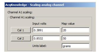
Channel scaling box with 20 g and 50 g scaling values
