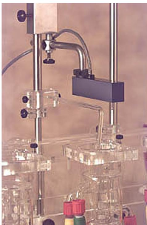
Forces are transmitted back to the beam via a self-centering pull-pin to insure accurate force measurements. The cantilever beam is mounted in a sealed aluminum enclosure which includes a 3/8" diameter mounting rod for holding the transducer in a large variety of orientations.
