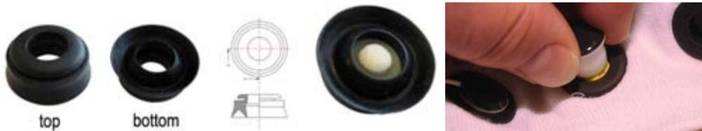
The sensor housing can contain a sponge that is soaked with water. The sponge and the water make contact with the skin to measure EEG. In order to increase comfort and decrease motion artifacts, the sensor housing is inserted in a rubber carrier, integrated into a type of headcap. The rubber ring prevents the sensor from drying out quickly and, more importantly, prevents sensor movement with respect to the skin. The carrier is produced from a soft type of rubber, and is very comfortable to wear.
