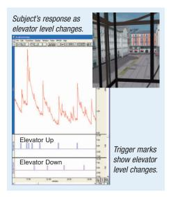
Use a feedback loop for greater control and automation of the VR world. This allows the world to change in real time, based on the subject's responses. Timing events are used for analysis of the physiological data.
