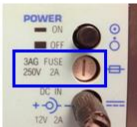
Location of fuse holder, back of MP160
