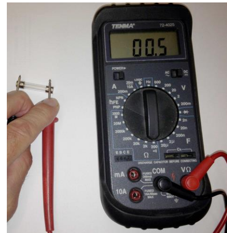
Testing fuse with digital multimeter
