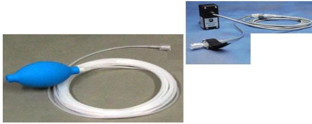
The TSD114-MRI consists of a pump bulb (RXPUMPBULB-MRI), pressure transducer (TSD104A equivalent, terminated in DSUB9), and tubing (AFT30-XL). Subjects can squeeze the bulb by hand or apply pressure via foot, thigh, etc. to indicate a response while in the MRI.
