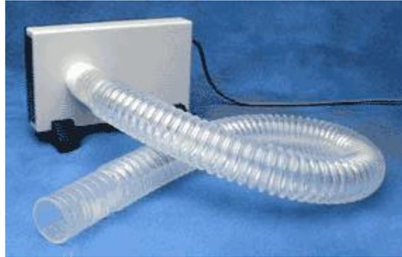
The TSD107B is a highly linear, wide range, airflow transducer. Using the TSD107B and a DA100C amplifier with the MP System, a variety of tests relating to airflow and lung volume can be performed. With the equipment listed below and the proper software parameters, precise lung volume measurements can be obtained.
