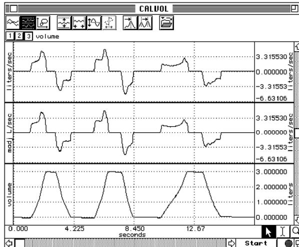
1. Insert a three-liter calibration syringe into the free end of the airflow tube.
