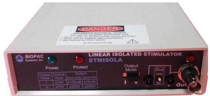
**Isolation characteristics**—The STMISOLA isolates the Control Input Voltage from the stimulus output to 1500 VDC HiPot and approximately 1000 pF of coupling capacitance.
