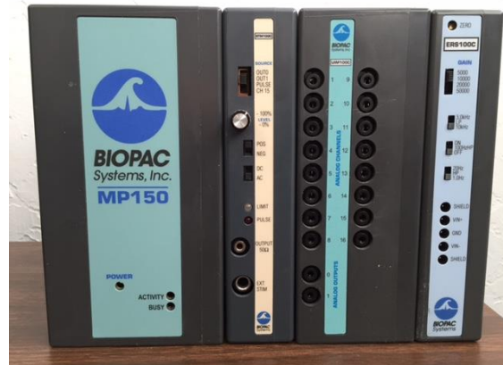
STM100C connection to MP device, UM100C and ERS100C
