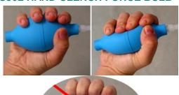
SS56L measures proportionality of bulb pressure to clench force in "kgf/m^2" units (a pressure unit). This measure is accurate for the relative measures recorded in BSL Lesson 2 Electromyography (EMG) II. SS56L is recognized by current release BSL Lessons.
