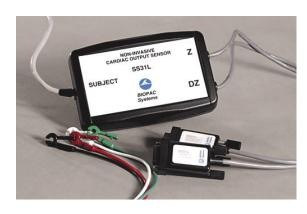
impedance of the tissue volume. The SS31L outputs impedance (Z) and derivative of impedance (dZ) in real time. Best used with BIOPAC $\alpha$  EL506 Bioimpedance strip electrode.
