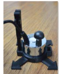
Diffuser unit with water level sensor
