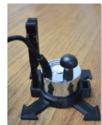
Diffuser unit with water level sensor
