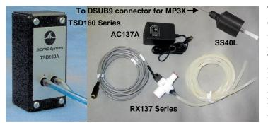
The TSD137/SS46L-SS52L series pneumotachs can be used to perform a variety of small animal and human pulmonary measurements relating to airflow, lung volume and expired gas analysis. These pneumotach transducers consist of a low flow, pneumotach airflow head (RX137B through RX137H and SS46L through SS52L) coupled to a precision, highly sensitive, differential pressure transducer (TSD160A or SS40L) via RX137 tubing. The pneumotachs will connect directly to a
