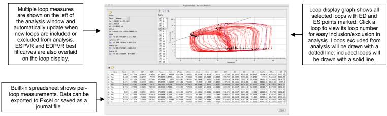
Full Pressure-Volume Loop Analysis Window with graphic loop display, multiple loop statistics, and built-in spreadsheet with per-loop measurements!
