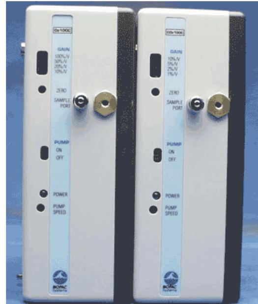
Both modules are equipped with a variable speed pump to adjust the flow over a wide range of sampling conditions. Sampling line connections for input and output flow are readily accessible on the front panel of either module.
