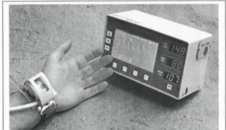
The analog output signal provides one output pulse per measurement cycle. The measurement cycle is updated every 10-15 beats of the heart.
