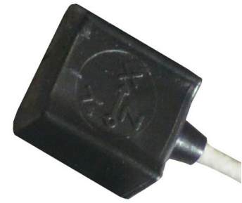
Tri-axial accelerometer uses 3 channel inputs
