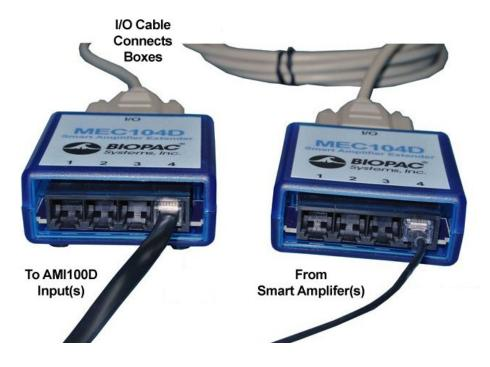
The MEC104D Smart Amplifier Extender provides a three-meter extension cable for up to four Smart Amplifiers. It consists of two extension boxes, one 3-meter I/O cable connecting the two extension boxes, and four RJ12 connection cables. One extension box connects up to four RJ12 cables to input channels of the AMI100D; up to four Smart Amplifiers plug into the other extender box. Multiple MEC104D extenders may be used simultaneously with an AMI100D.
