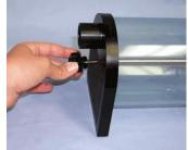
2) Remove the plastic lid from the flow chamber.
