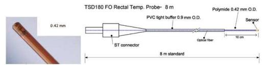
• The Polyimide round tubing protects the sensing element its flexibility and rigidity provide excellent pushability.
