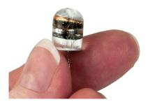
EPOCH differential sensors enable wireless recording of two different biopotentials with their own reference.
