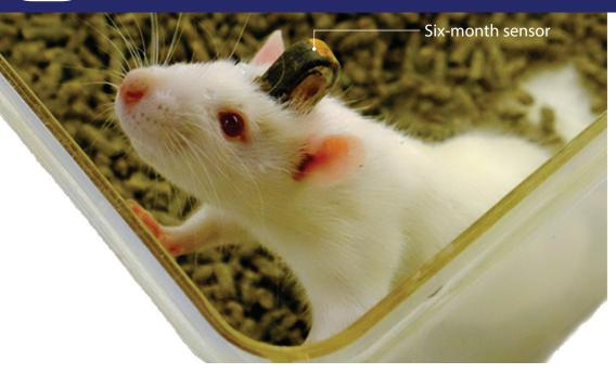
EPOCH sensors record up to six channels of wireless biopotentials with high signal-to-noise ratio for up to six months from rats and mice — even pups!
