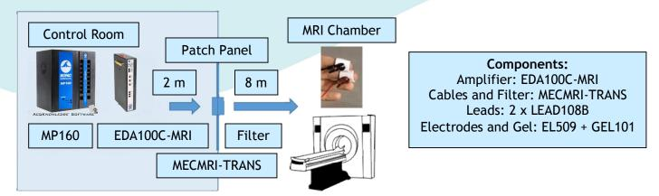
BIOPAC MP160 Research System with EDA100C-MRI Amplifier Module cabled for MRI environment
