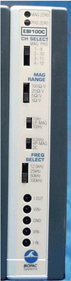
The EBI100C records the parameters associated with cardiac output measurements, thoracic impedance changes as a function of respiration or any kind of biological impedance monitoring.
