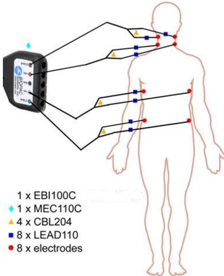
**NOTE:** The EBI100C measures bioimpedance in terms of both magnitude and phase as a function of frequency (12.5, 25, 50, and 100 kHz). The choice of interfacing cables will impact both magnitude and phase readings. The impacts will be larger as the frequency of the source current increases. To obtain accurate measures at any frequency, calibrate the measurement for magnitude and phase after the interface cabling infrastructure is stabilized. (See EBI100C Calibration steps on page 4.)
