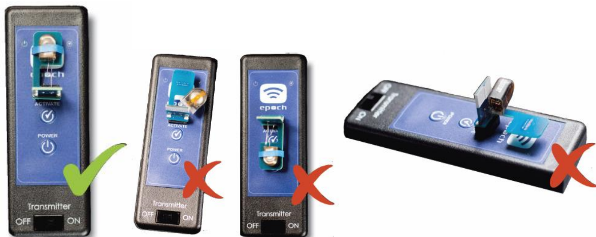
Figure 14. Proper placement of Sensor in Activator/Tester shown on left
