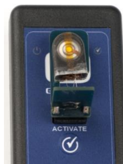
Figure 13. Activation of dual channel sensor shipped in off state
