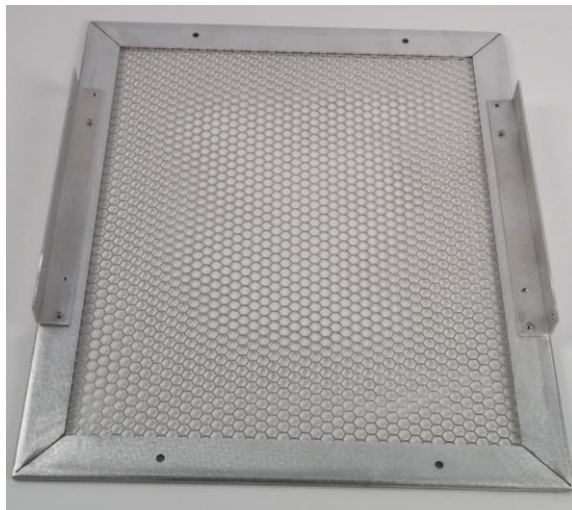
Figure 22. Step 1 – Top assembled using one long panel and two L-brackets
