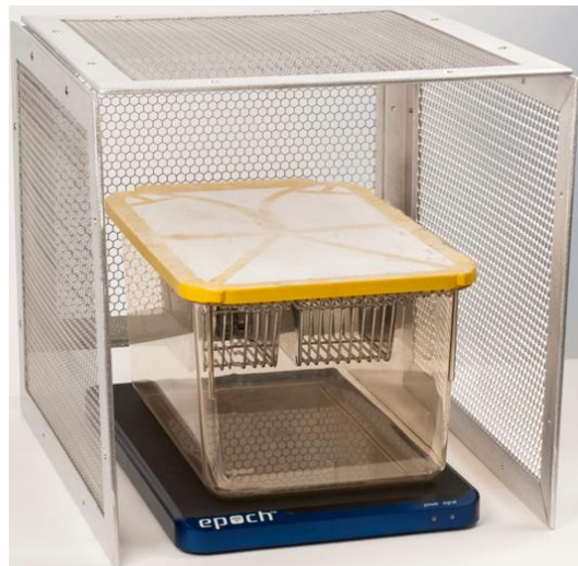
Figure 17. Completed Faraday shield assembly
