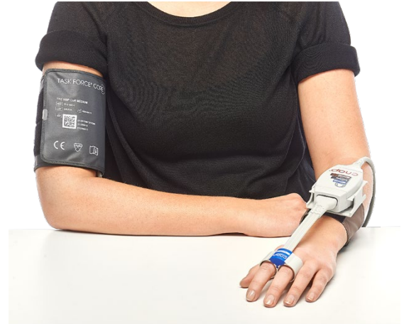
Properly positioned finger cuff controller and sensor
