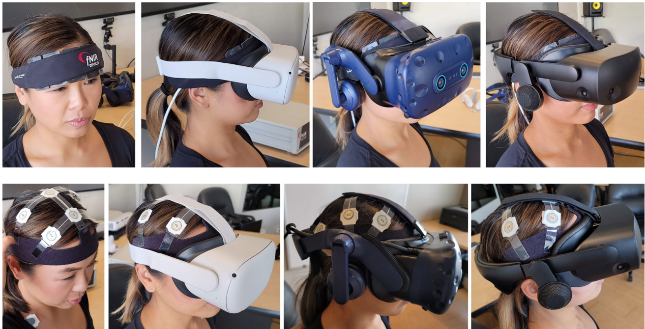
fNIRS (top, left) and B-Alert X-Series EEG (bottom, left) sensors were tested for comfort and functionality when used in combination with three popular VR HMDs: (left to right) Oculus Quest 2, Vive Pro, and HP Reverb.
