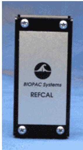
The **REFCAL** is used to check the reference voltage of the **DA100C**. It connects to the DA100C and displays the reference voltage as an analog input signal. This makes it very easy to adjust the reference voltage of the DA100C to suit the transducer.
