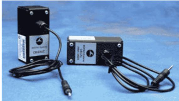
**CBLCALC** Calibration Cable for 100C-series Biopotential Amplifiers.
