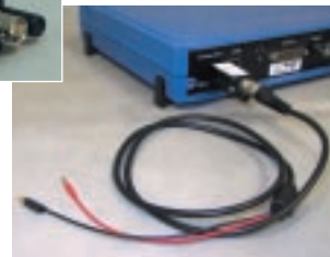
SS58L connected to MP35 with BSLCBL2A.
