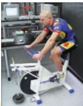
Ergometer modified to record WAnT using BIOPAC
