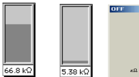
MP30 Poor contact MP30 Good contact MP30 Off
