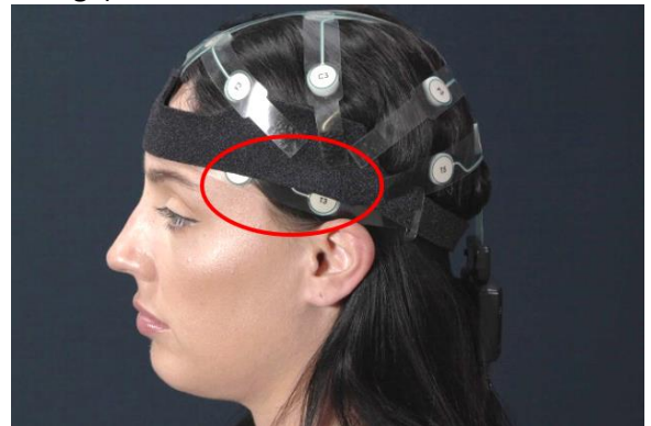
18. Riding up of the Headstrap where the Strip is revealed may be caused by too small of a Strip, or aggressive tugging during troubleshooting.
