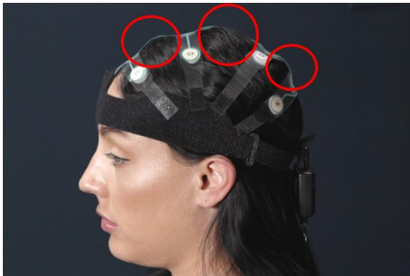
17. The buckling shown in the red circles can be caused by not keeping the Strip taut from front to back, or an incorrect strip size.
