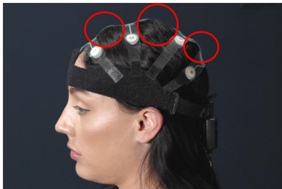
15. The buckling shown in the red circles can be caused by not keeping the Strip taut from front to back, or an incorrect strip size.
