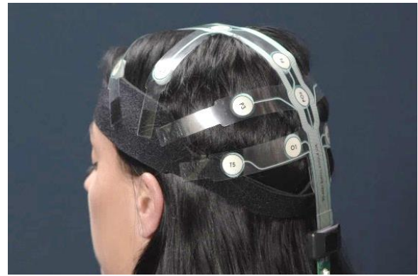
12. While troubleshooting, be careful to maintain the correct alignment of the Strip on the scalp, ensure that the Strip is lying flat without any creases, and that the foam donuts are slightly compressed.
