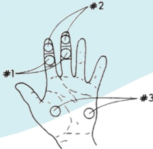
Three electrode hand placements for recording electrodermal activity.
