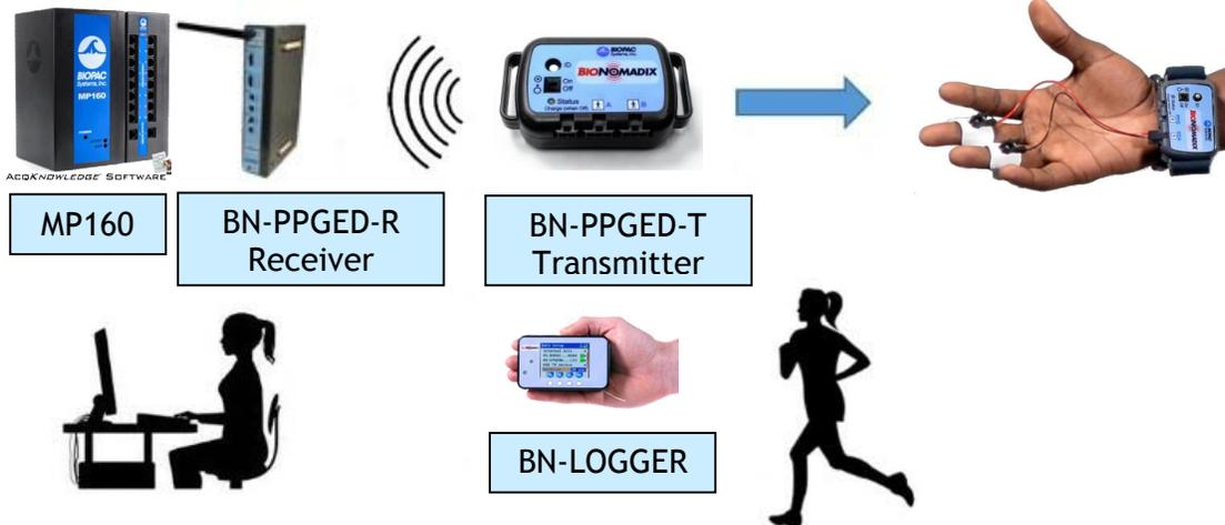
*BIOPAC MP160 Research System with BioNomadix Receiver, Transmitter, or BioNomadix Logger*
