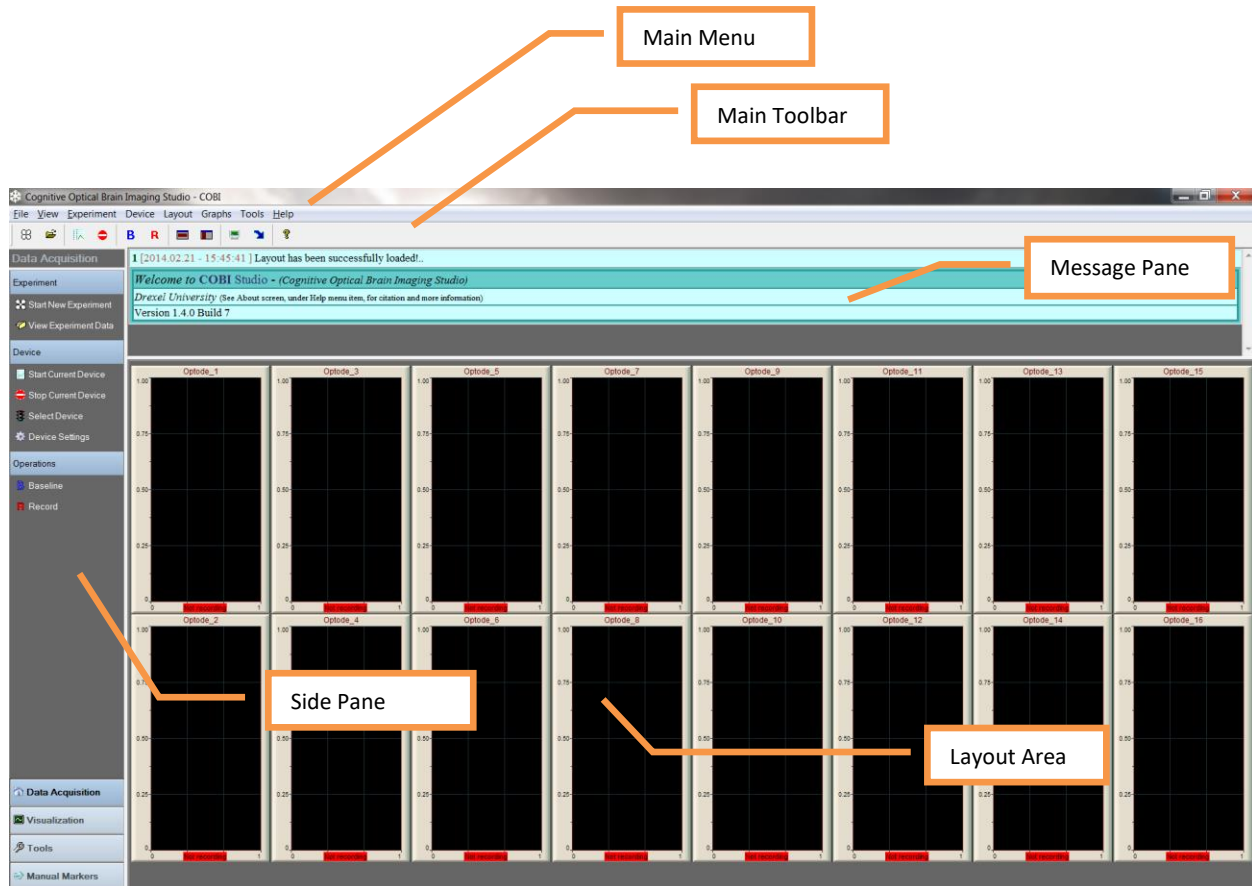
Figure 4. COBI main window and components
